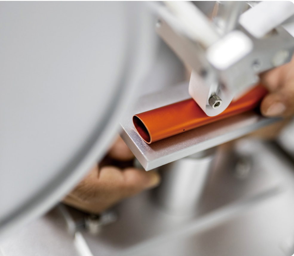
The RLX Tech’s product during the paper-tape friction test in the Quality and Safety Testing Laboratory.
